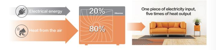
Prior to this, traditional heating systems mainly used fuels such as gas, oil, and coal but these fuels easily cause environmental pollution, emit large amounts of carbon dioxide into the air, and cause global climate changes. The air source heat pump system effectively reduces environmental pollution while maintaining high energy efficiency.
