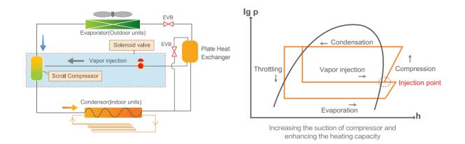
The vapor injection system and stepless inverter technique greatly improve the refrigerant cycle system. It effectively increases refrigerant flow through vapor injecting, thus substantially enhancing the heating capacity.
